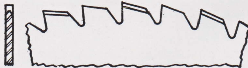
COPPER SLITTING TOOTH — each alternate tooth is "V" shape on top
